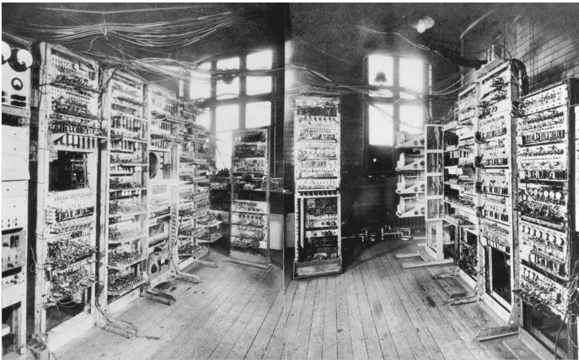
Babbage, Charles The realization of Babbage's dream: the Manchester Mark 1 computer at Manchester University, England, in 1948. This was the first computer that could store both data and programs electronically. Ferranti Electronics Ltd.
